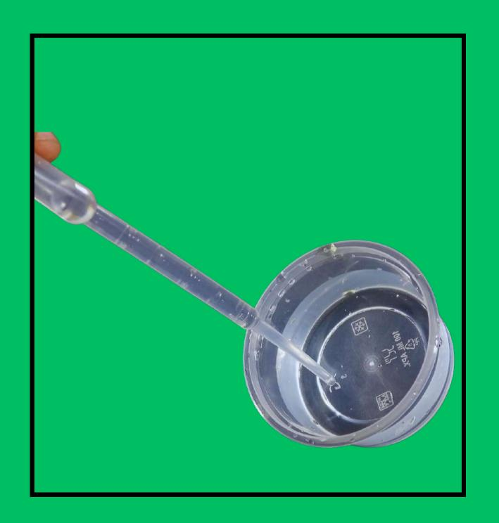
Carefully squeeze out water drop by drop from the pipette onto the coin. Count how many drops fit on the plate before the dome breaks and the water spills over
