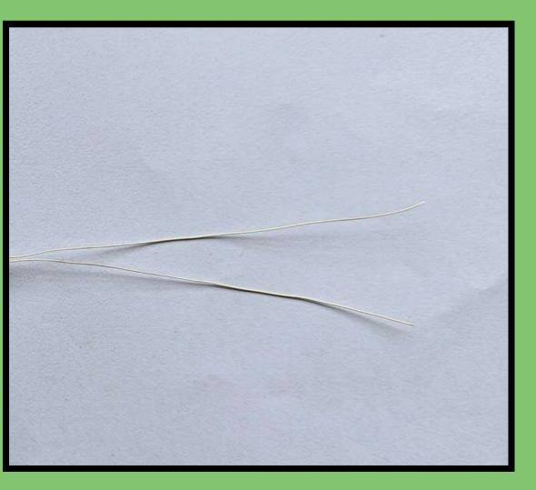
NOTE - Before connecting the LED in the circuit, check whether the LED's long wire ends are burned or scarred. They should be black in color. If they are still coated with a golden color on both ends, rub or scratch them using scissors or any rough surface material as shown.
